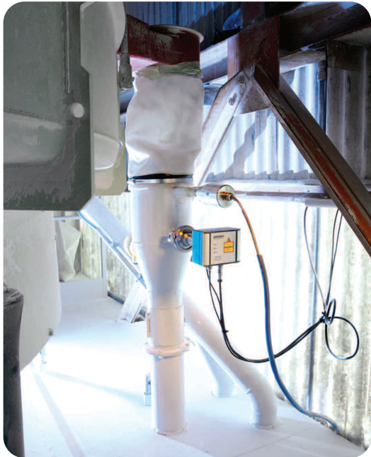
☛ The particle size analyser was installed on the exit line from a sieve stack at Ferrari Granulati
